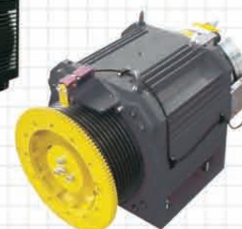
MRL GEARLESS PERMANANT MAGNET TRACTION MACHINE
